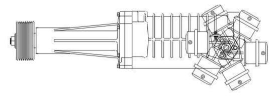
Actuator can mount in any one of 12 possible positions with 6 on each side.
