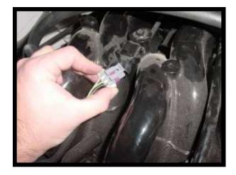
Idle Air Control (IAC) connector. Squeeze and pull to remove connector.
