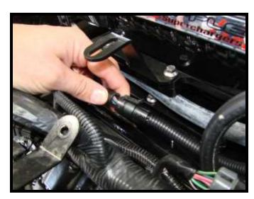
Plug in male end of TPS extension into new TPS sensor on port side of throttle body.
