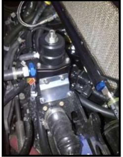
Picture is an example of remote mounting regulator
