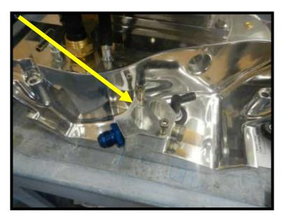
23. Utilize the factory reusable intake gaskets, install against head. Make sure to read (this side down) on the bottom of each for proper installation. Replacement gaskets are available through Whipple or your Mercury Marine dealer if gasket is damaged.
