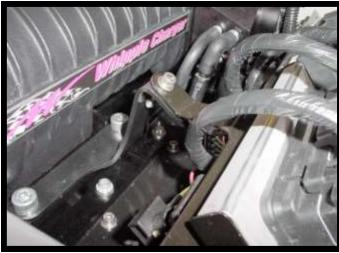
45. Adjust fuel pressure, VERY IMPORTANT, MOTOR WILL NOT IDLE IF SET INCORRECTLY.
