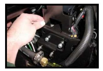
21. Install new supplied NGK BR7EFS spark plugs. Proper plug gap is .035", check and verify each plug. Reinstall factory plug wires.
