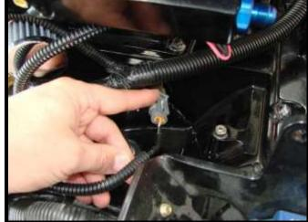
Connect the supplied 2-bar map connector pigtail to factory wiring connector. Verify that the color wires match the pins. Plug the new 3-way round connector into new MAP sensor installed at port side, rear of engine.
