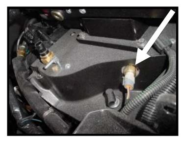
Install factory IAC motor to the billet adapter located on the back of the intake manifold. Utilize the new supplied gasket between the two surfaces. Secure with the supplied ½" x 2" socket head allen bolts. This will only mount one way.
