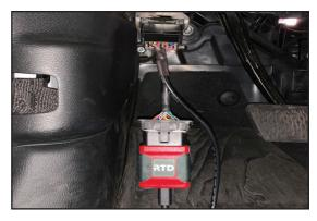
For 2012-2017 vehicles plug the RTD directly into the ODB port.
