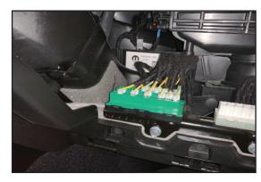
11. Take the supplied bypass cable and connect the white connector as shown at the red arrow location. Route the cable along the base of the dash towards the OBD connector. Use zip ties to secure it out of the way.
