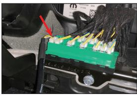
12. Plug the end of the supplied connector into the ODB port. (The other end will be used when flashing with the RTD device.)
