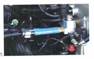
68. Re-attach the circlip to retain the regulator.
