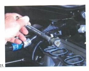
24. Remove Intake Manifold.
