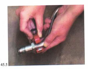
45. Since the EGR Valve has been re-located, the EGR Tube must be "Modified". This can be done with common hand tools. (shown Sears 51252 tubing cutter) The tube must be cut in two (2) places and mended with brass crush collars on the end of a flexible stainless steel tube.
