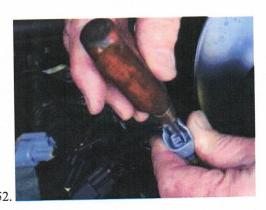
51. The injector plugs need to be swapped to match the 30# injectors. Disassemble the connectors as shown. Cut and strip wires. Crimp terminals to wires and insert into new connector. Be sure not to reverse the polarity of the wires. (red wire to left as installed into injector) Swap all 8 injector plugs.
