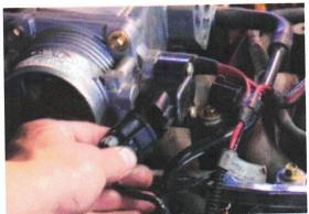
5. Disconnect vehicle wiring harness connectors from ignition coils; throttle position sensor, idle air, EGR solenoid valve, EGR Pressure Transducer, Temperature Sensors, fuel pressure, and fuel injector connections.
