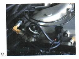
64. Re-attach the throttle and cruise control cables and return spring. Check for proper operation and adjust cruise cable attachment if
