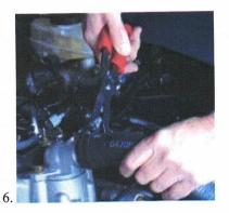
15. Disconnect water heater hose from intake manifold.
