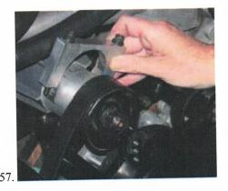
56. Install alternator bracket to front of engine, hand tighten the bolts. The belt must be routed properly before attempting this step. Refer to Figure 2. (P13.) for belt routing.
