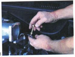
23. Remove thermostat housing, thermostat and O-Ring from the Intake manifold.
